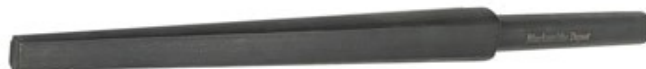
4140 Hammer Eye drift 15" total length 10" of tapered drift area 5" tong holding area - approx. 7/8" round Tapers from approx 7/16" x 5/8" to 1" x 1-1/4"
